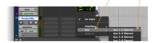
4e. The output of the Aria player is now routed internally to the input of Rudolph Mix.
